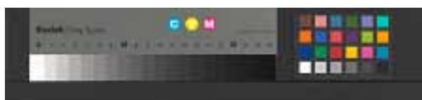
Because a Q-13 exists in every image the tonal capture can be assessed at all times. And because a mini ColorChecker is on the right side of the Q-13, illumination in the frame of the Q-13 image can be assessed. Thanks to the mini ColorChecker neutrals the white balance too can be assessed.
